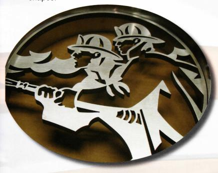
Abrasive Water Jet is excellent for the cutting of complex shapes, and in fragile materials such as glass, the high failure rate due to breakage and chipping of corners during conventional processing is virtually eliminated. Whatever your industrial need, Abrasive Water Jet is an accurate, flexible, and efficient cutting system.
